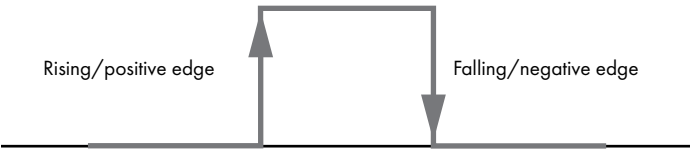
Figure 6-12: Pulse edges illustrated
